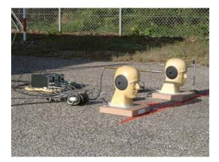
Figure 10. Experimental set-up for attenuation measurements with impulsive noise at ISL.
