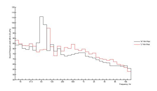
Figure 7 Cockpit noise in the C130K and C130J variants of the Hercules
