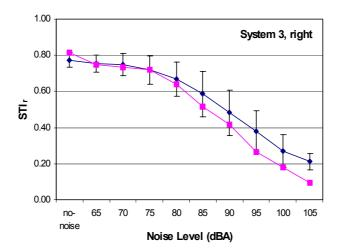
Figure 19. STI<sub>r</sub> as a function of the background noise level for system 3 (right earcup).
