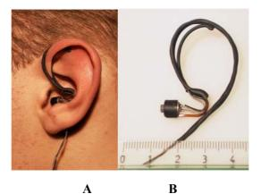
Figure 5. Microphone configuration used for the MIRE-method.
