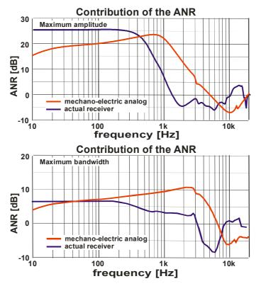
**Figure 30:** Contribution of ANR in an active earplug with an actual receiver (blue) or the electro-mechanic analog (red)
