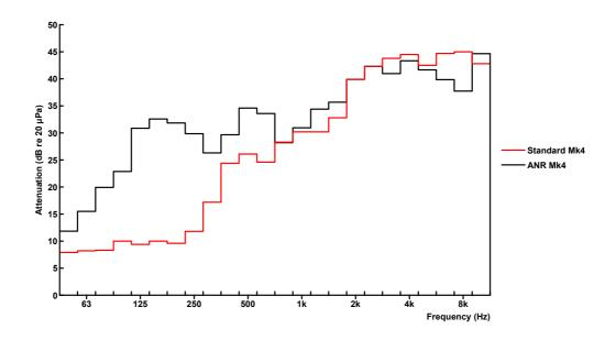
Figure 11 The passive plus active attenuation performance afforded by a helmet mounted ANR system
