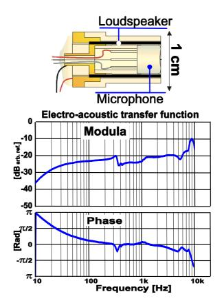
Figure 26: Piezo-ceramic ANR earplug and its electro-acoustic transfer function
