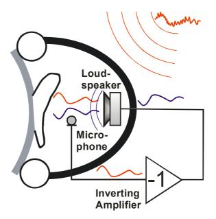
Figure 6: Basic principle of ANR using feedback control
