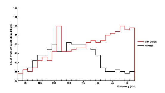
Figure 3 A comparison of cockpit noise in the F-16A with ECS switched on and off
