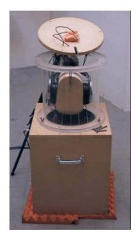
Figure 8. Dummy head with "flat-plate" microphone in a volume suitable for relatively high noise levels (130 dBA).
