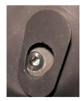
Figure 6. Artificial ear mounted in an artificial head (MIArtE).
