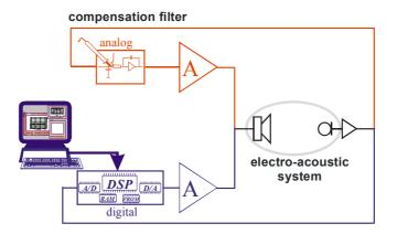
Figure 12: Analog (blue) and digital (red) controlled ANR system
