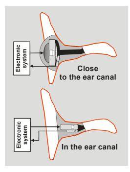
Figure 25: "Close to the ear canal" and "in the ear canal" position of the transducers in an active earplug
