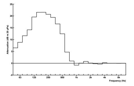
Figure 10 The active attenuation performance afforded by a helmet mounted ANR system
