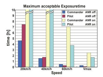
**Figure 18:** Maximum exposure times at different places (commander or pilot) and for different running conditions of the tank when using active or passive hearing protectors.
