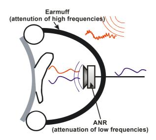
Figure 4: Principle of ANR underneath an earmuff
