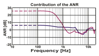
Figure 28: ANR of an active earplug using "hearing aid"-type receivers
