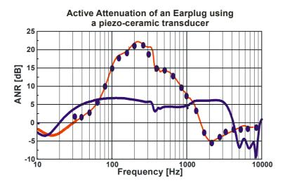
Figure 27: ANR earplug using a "hearing aid"-type receiver and the electro-acoustic transfer function of the system
