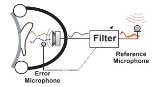
Figure 5: Principle of a feed forward control
