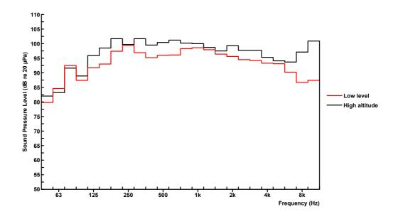
Figure 4 A comparison of cockpit noise in Jaguar during high and low altitude flight
