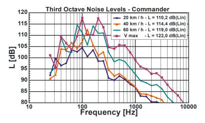
Figure 1: Typical noise inside an armoured vehicle
