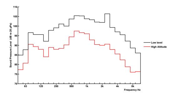
Figure 2 A comparison of cockpit noise in Harrier during high and low altitude flight
