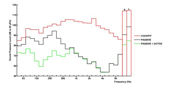
Figure 12 A comparison of noise levels at the ear in Harrier GR5 during high-speed low level flight for passive and passive plus active helmet attenuation.
