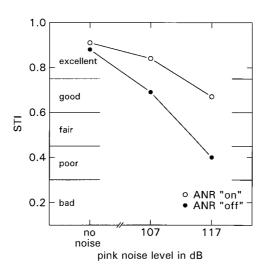
Figure 17 STI at three noise levels for an ANR system switched on and off.
