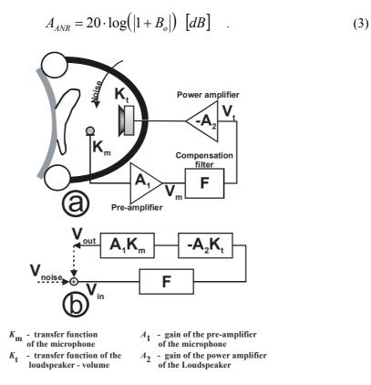
**Figure 7:** (a) Different electrical and electro-acoustical elements of the ANR system. (b) Equivalent block diagram of the opened (solid line) and closed (solid + dotted line) feedback loop
