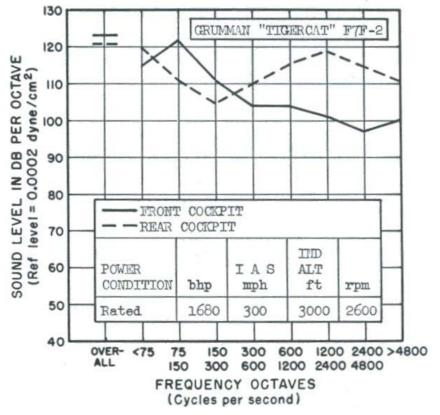
Figure 1 Cockpit noise in F7F-2
